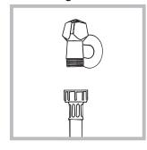
1. Connect the supply pipe by screwing it to a cold water tap using a 3/4 gas threaded connection (see figure). Before performing the connection, allow the
